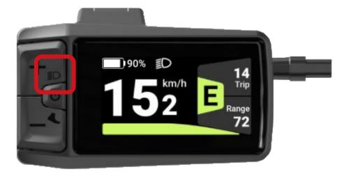
■ Note: When your e-trike is powered on, the throttle remains disabled until you switch the Power Assist System (PAS) mode from Off to Eco, Tour, Sport, Sport +, or Boost mode.
